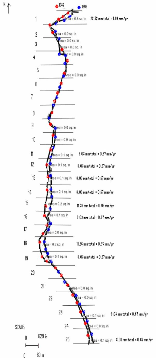
**Figure 1: Shoreline outlines.** The photographs were blown up to a scale of 1:5000. One inch in the photograph represents five thousand inches in real scale. (1 in = 0.0254 m; 80 m = 3,149.6062992 in (real scale); 80 m = .629 inches (Aerial Photo)).
