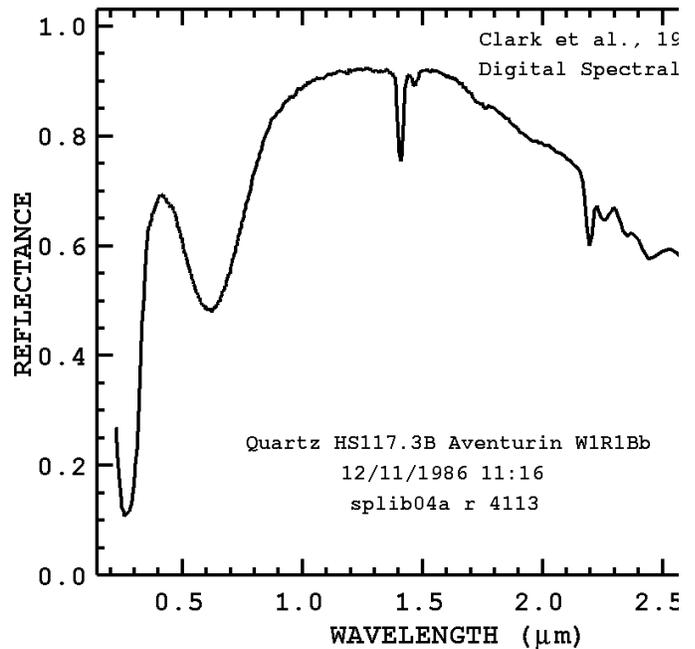
Figure 6. U.S. Geological Survey by a field measurement for Quartz.
