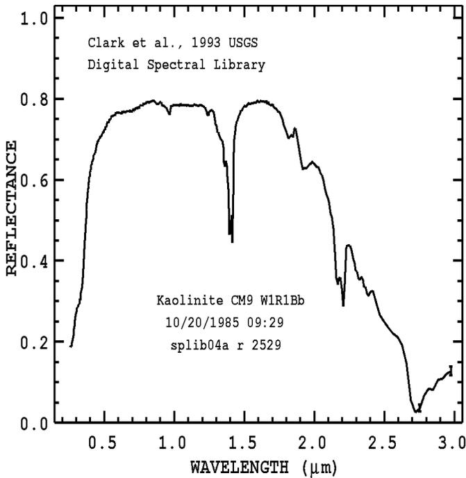
Figure 8. U.S. Geological Survey by field measurements for Kaolinite.
