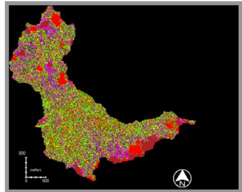
**Figure 6. Unsupervised Isodata, (6) classes, (2) maximum iterations, convergence threshold 0.950**
