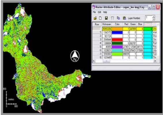
**Figure 8. Supervised Minimum Distance Method, using training samples.**
