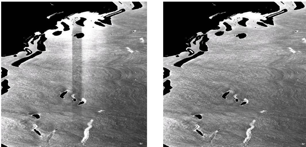
Figure 3: Original subset image with central stripe (left) and after halo suppression (right).
