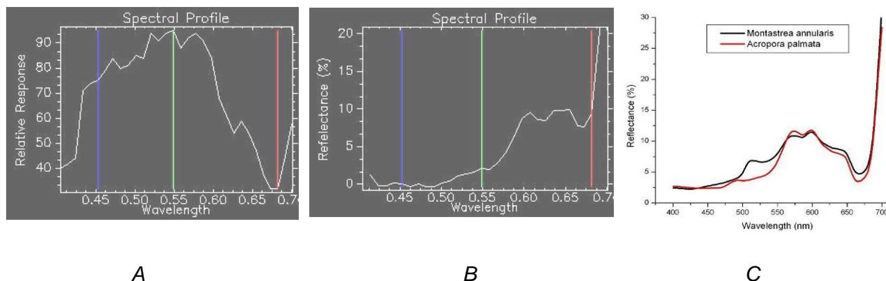
Figure 6: AVIRIS coral spectrum without water column correction (A) and after the correction (B). Representative field spectra from two species of corals is shown for comparison (C).
