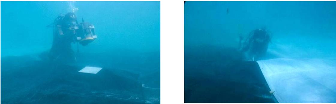
Figure 2: The dark (left) and bright (right) underwater calibration tarps at Enrique Reef.
