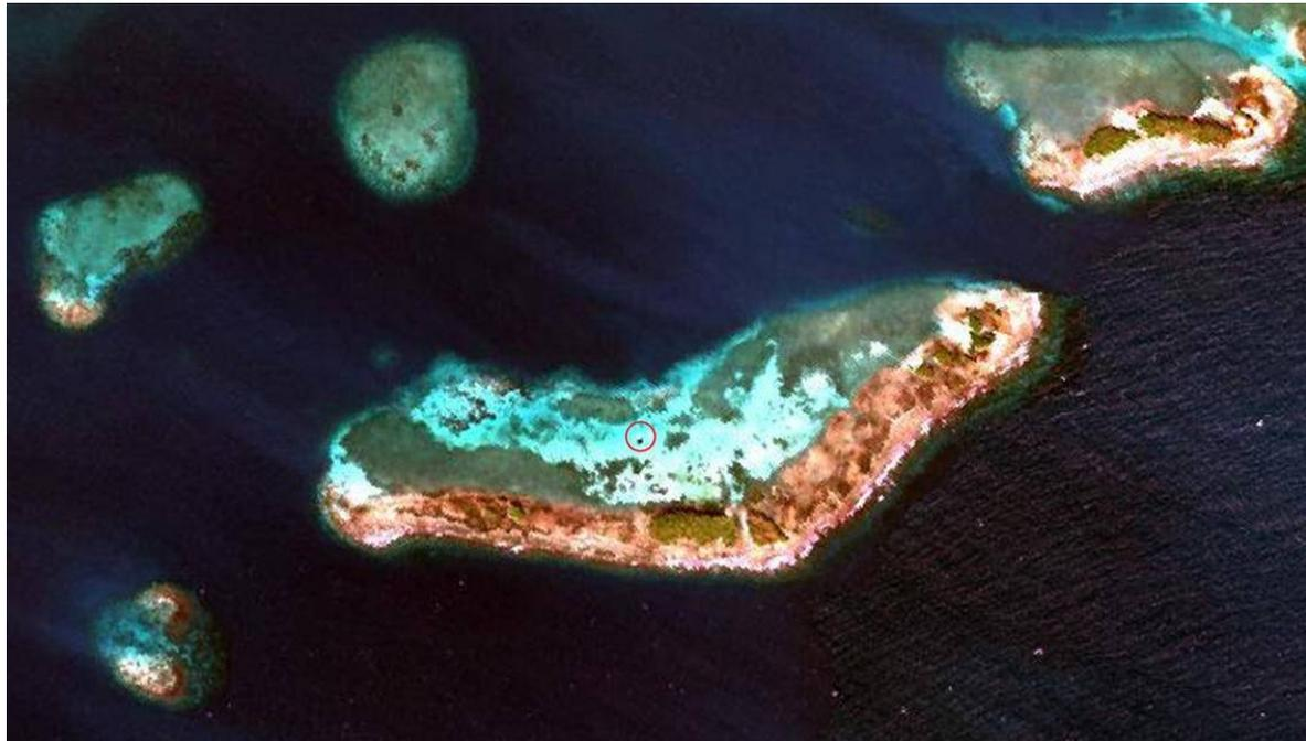
Figure 4: AVIRIS subset of Enrique Reef and adjacent reefs after water column correction. The white and dark pixels within the central oval are the underwater calibration tarps.
