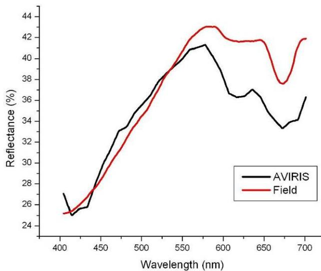
Water column correction validation using a sand target.
