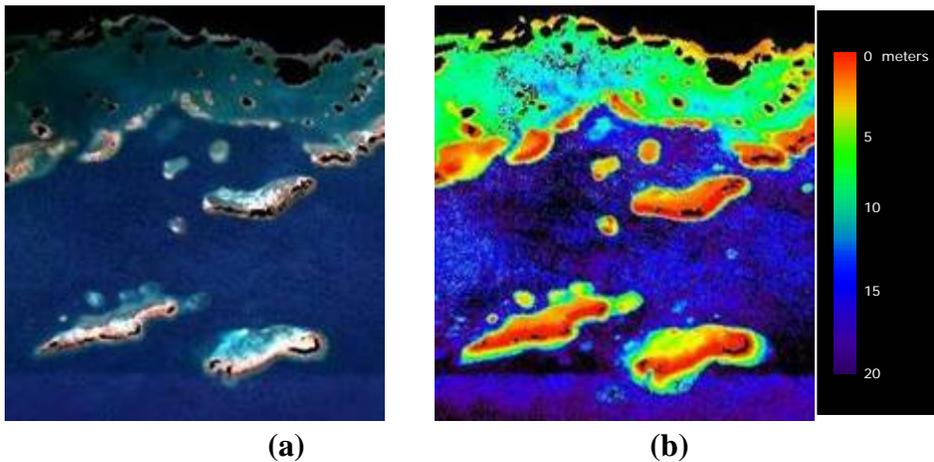
**Figure 6: AVIRIS color composite with land mask (a) and estimated bathymetry after image processing (b).**
