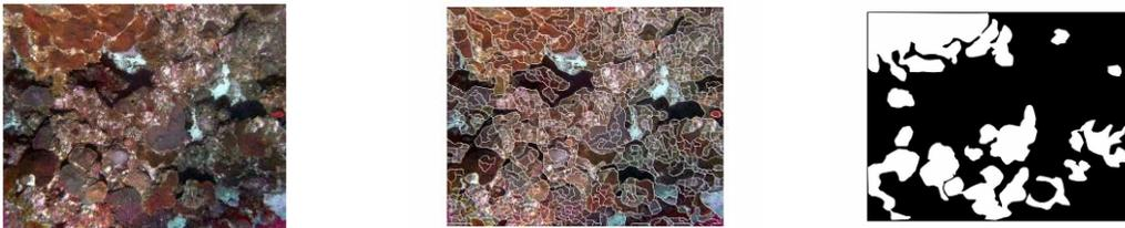
**Figure 9:** (a) Original image, (b) Enclosed areas are the result of segmentation using the LHC method, (c) Binary image classified using Canvas software.
