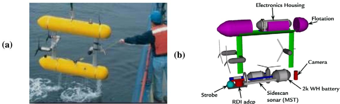
Figure 8: The Seabed AUV at the surface (a) and schematic diagram of the major components (b).
