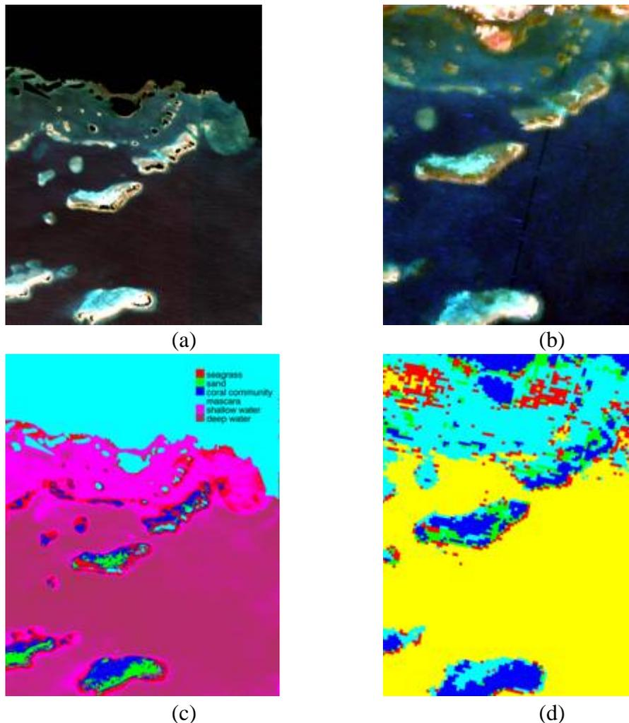
**Figure 4: Atmospherically corrected IKONOS (a) and HYPERION (b) and results of supervised classification of IKONOS (c) and HYPERION (d)**
