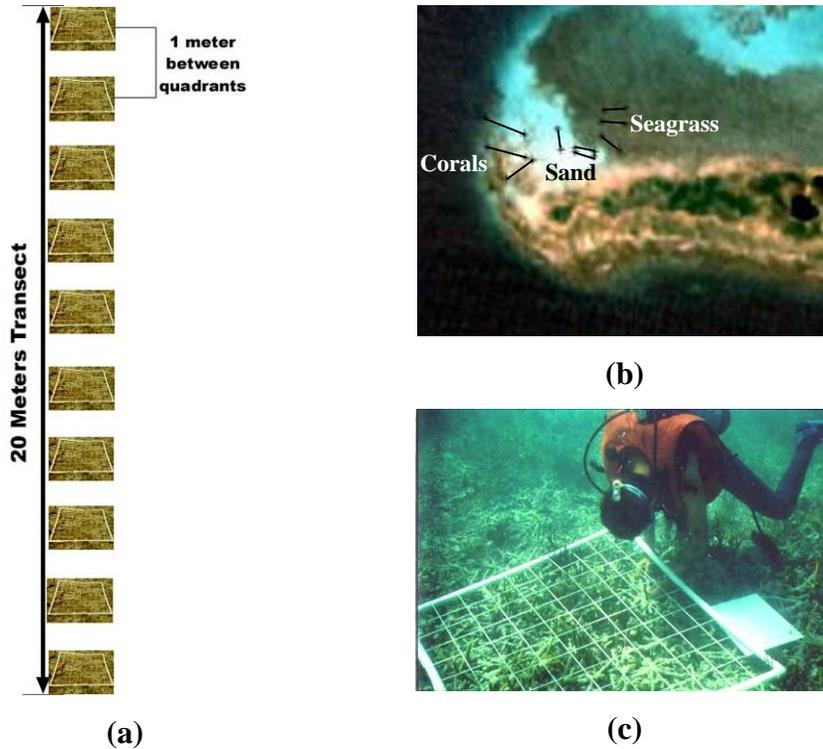
Figure 7: Field sampling at Enrique Reef. (a) Design of transects and quadrants, (b) IKONOS image showing the transect location according to bottom type in Enrique Reef, (c) Quadrant used to characterize bottom type.
