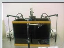
**INDOOR TANK:** It is composed of a small tank, light sources and hyperspectral imager and a spectrometer sensor. The hyperspectral imager consists of a 640x480 resolution CCD camera along with two tunable VariSpec filters. One filter covers the range from 400 to 720 nm, the other from 700 to 1100 nm. The spectrometer is a GER 1500 with a spectral range from 300 to 1100 nm and a FWHM of 2.8 nm. The primary light source for the tank are two halogen quartz lamps with fiber optic cables.
