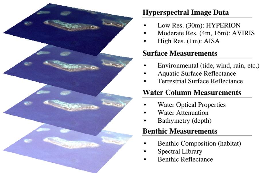
Fig. 1. SeaBED multiple level data collection concept.
