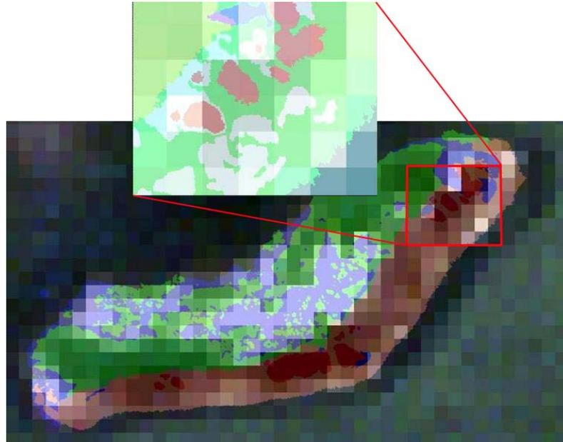
Fig. 6. Low resolution Hyperion pixels overlaid on high resolution basemap.
