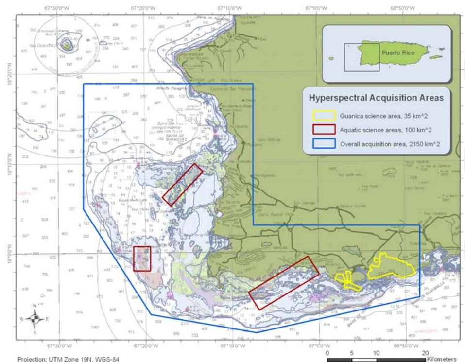
Fig. 2. Mission study area: blue polygon represents data at 4m GSD, red polygons represent science areas at 1m, 2m, 8m GSD and yellow polygons represent terrestrial science area at 1m GSD.
