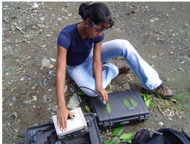
Figure 2. Measuring the reflectance of the leaves using the GER 1500 spectroradiometer.
