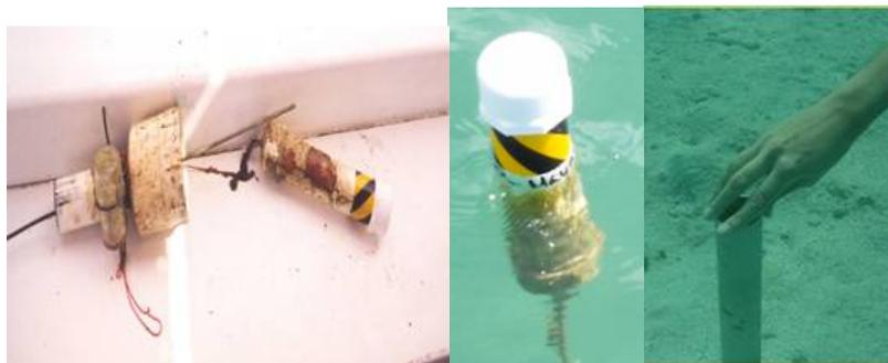
**Figure 3: Sediment traps used during this study.**
