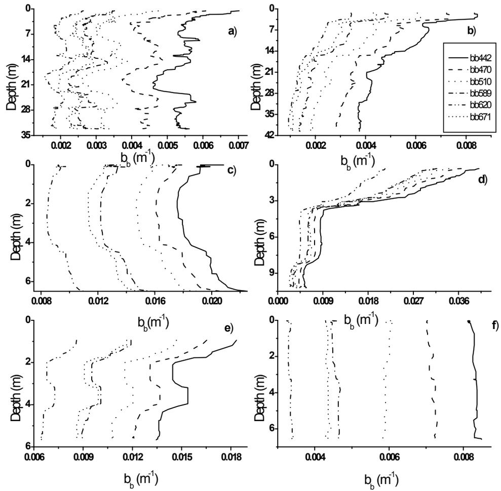
Figure 14. Profiles of the backscattering coefficient for Oceánica(a), Manchas (b), Atuneras (c), Añasco (d), Acueductos (e)and Rodríguez (f) in Mayagüez Bay during July 98. The legend at the top right corner applies to all graphs.
