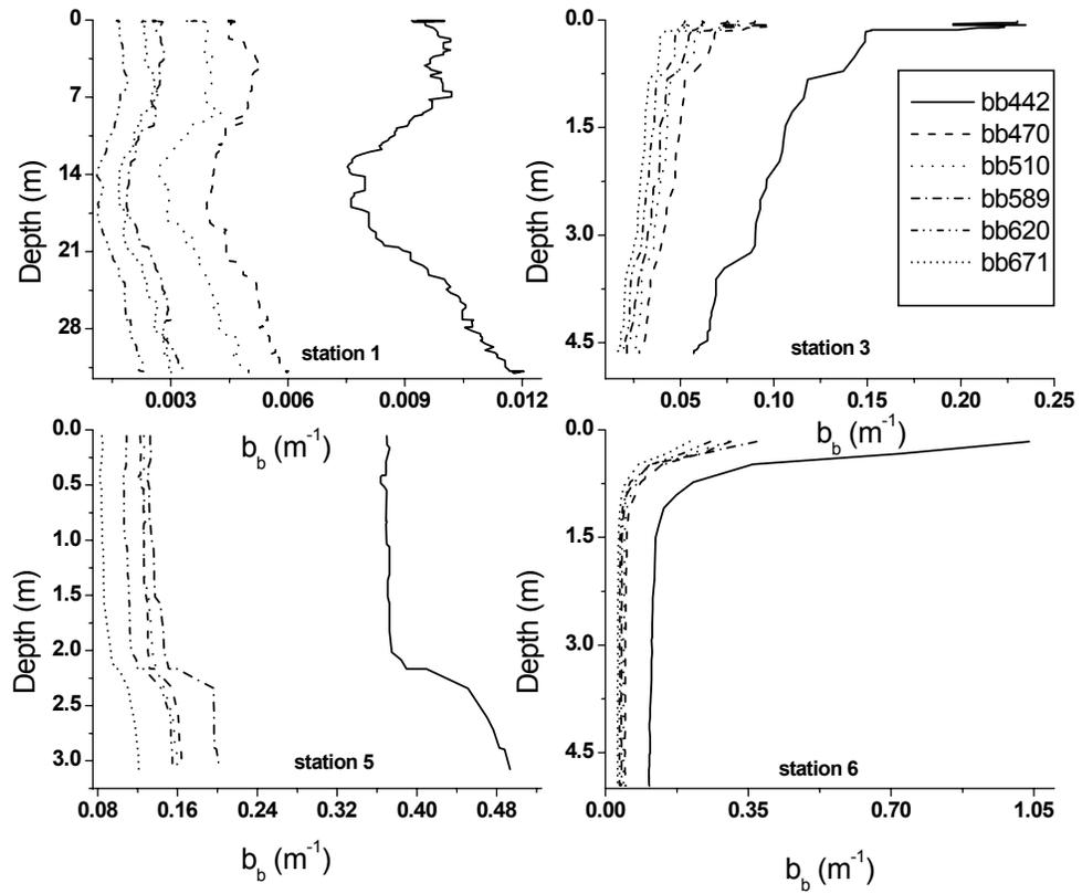
Figure 15. Profiles of the backscattering coefficient for selected stations in the Guanajibo River cruise, October 1998. The legend at the top right corner applies to all graphs.
