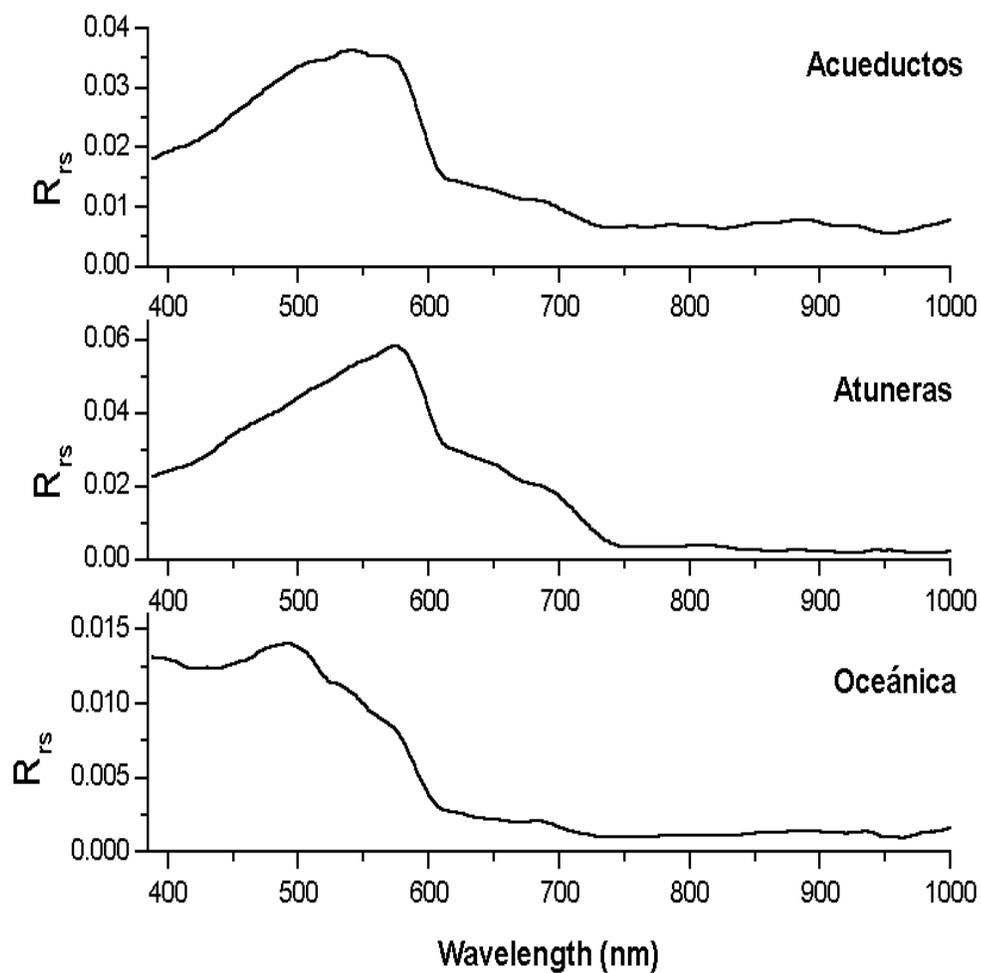
Figure 19. The three typical spectral shapes of remote sensing reflectance ( $R_{rs}$ ) curves obtained in Mayagüez Bay. These examples are from November 1997. Notice the difference in magnitudes of the y axis.
