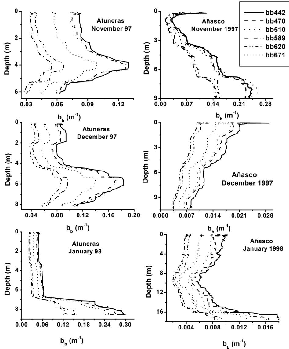
Figure 11. Profiles of the backscattering coefficient for Atuneras and Añasco stations for November 1997 (top), December 1998 (middle) and January 1998 (bottom). The legend at the top right corner applies to all graphs.
