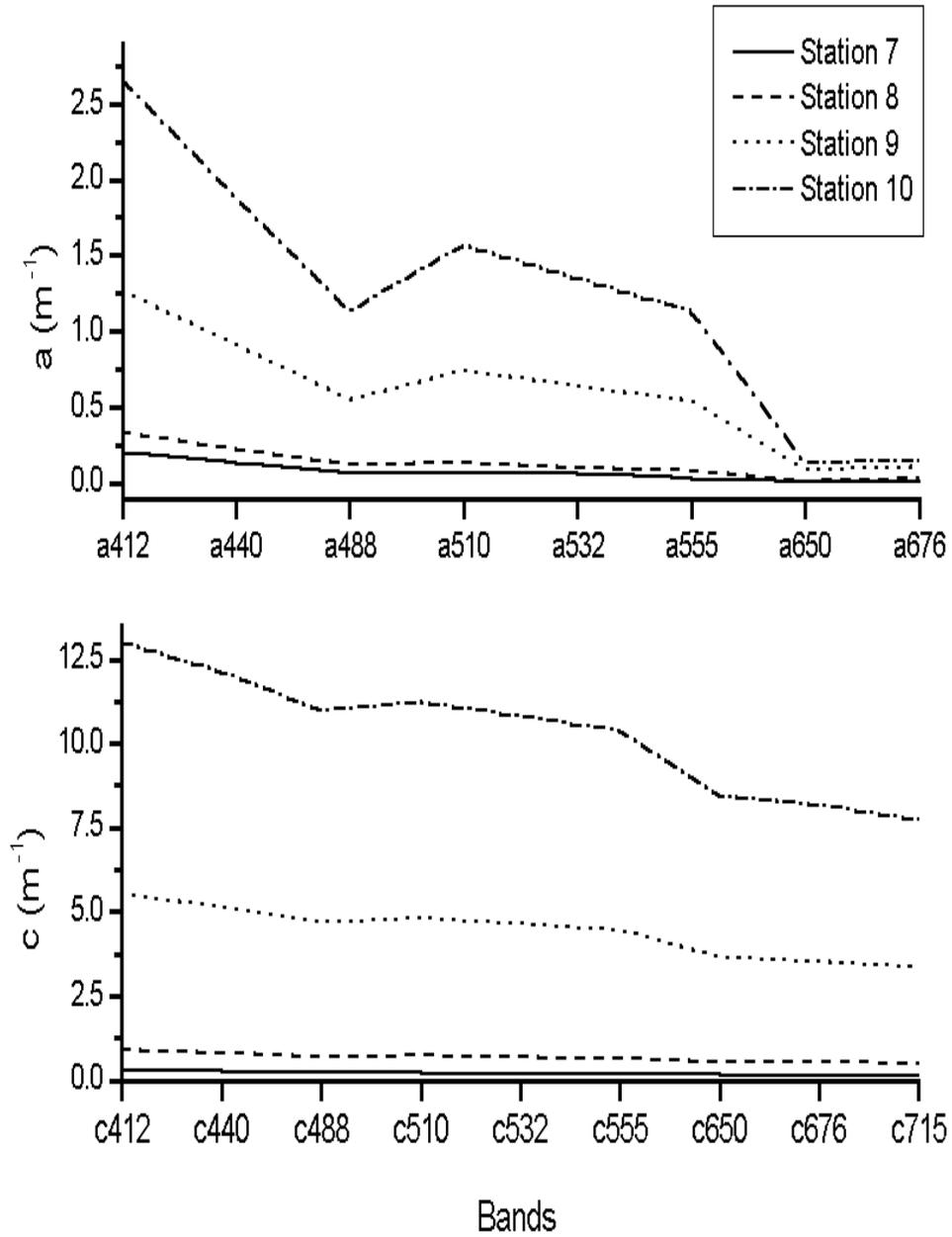
Figure 17. First meter average of total absorption coefficient ( $\text{m}^{-1}$ ) and beam attenuation coefficient ( $\text{m}^{-1}$ ), in Yagüez River stations, October 1999.
