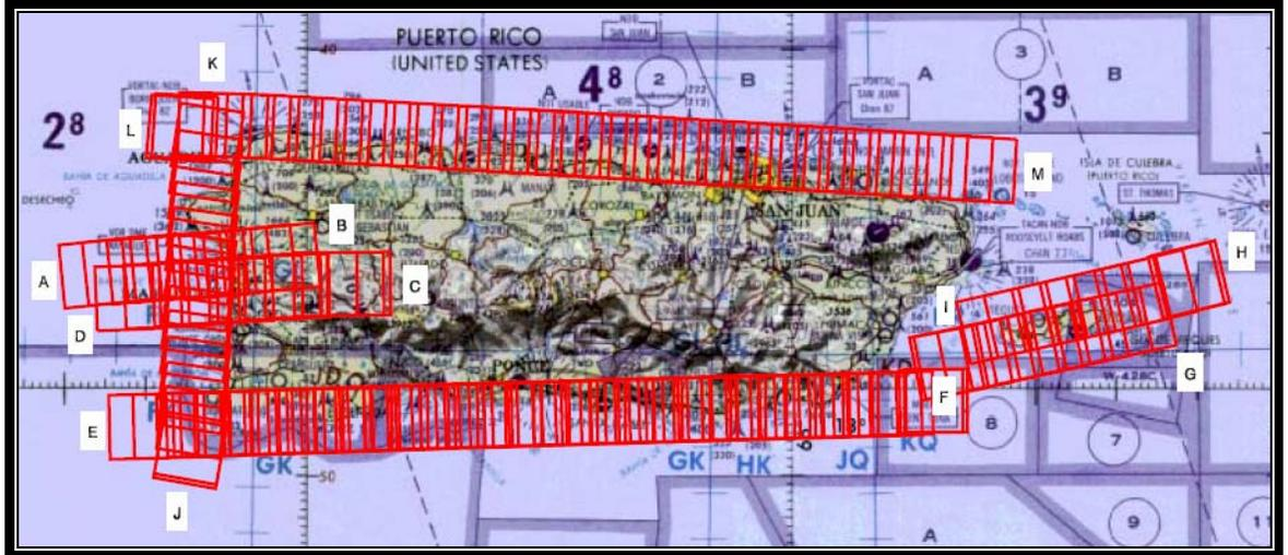
Figure 3: Map of Puerto Rico with six transects produced by AVIRIS sensor in August 19, 2004 (from Flight Summary Report Guild, NASA Research Center, 2004)
